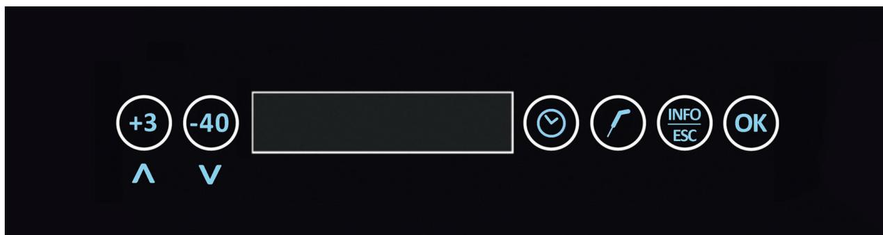
The models have a “Compact” power electronics board and “Glass” mechanical display. The user interface has a 6-digit LED scrolling display and 6 buttons:
